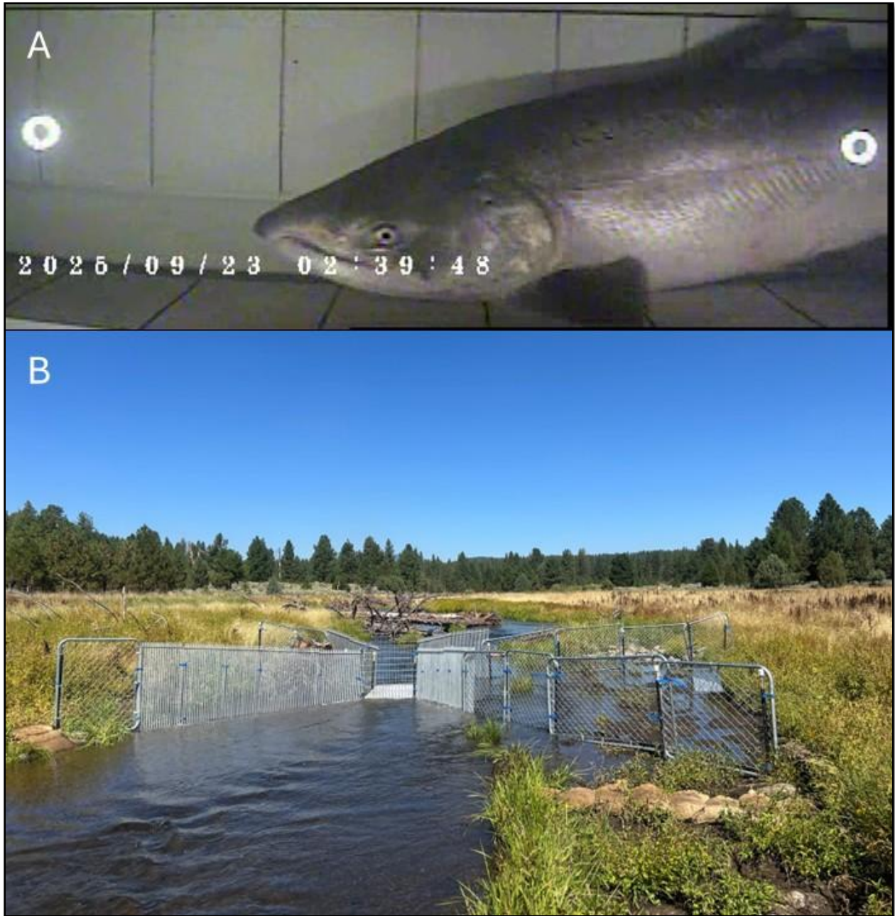
Figure 6. Photo of a fall-run Chinook Salmon in the fish chute at Spencer Creek Video Weir (A). And photo of Spencer Creek video weir (B).
